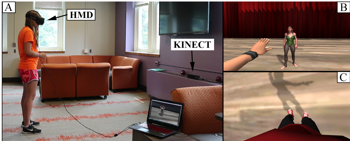
Figure 3.14: (A) The immersive embodied metaphor experiment setup with the head-mounted display (HMD) on the user's head, and a Kinect sensor in front of the user. (B) Screen capture of the virtual character that dances in front of the user. (C) The first-person view of the user's virtual body.
